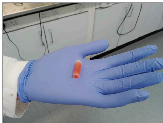
Figure 1 A hand-held PhLi gel cylinder ready for a reaction!
